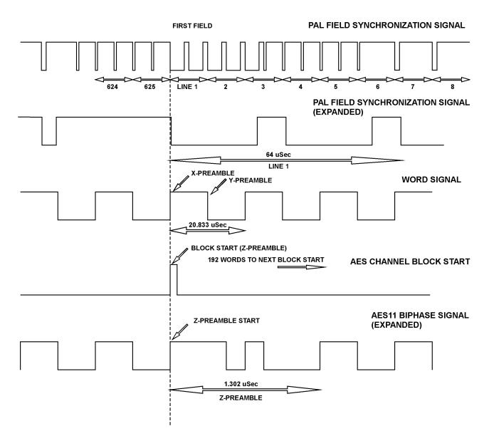
The generator places the video, word and AES block start as seen on the graphic representation above. At 48 kHz sampling frequency, the relationship is straightforward:
