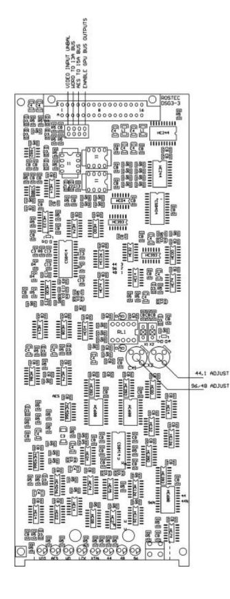
Jumper settings: Video jumper on: Unbalanced mode (default) Video jumper off: Balanced mode
