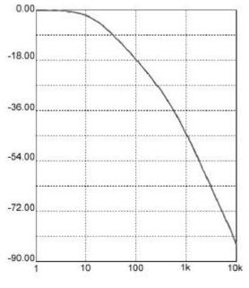
Jitter Attenuation dB vs. Frequency. AES input to AES output
