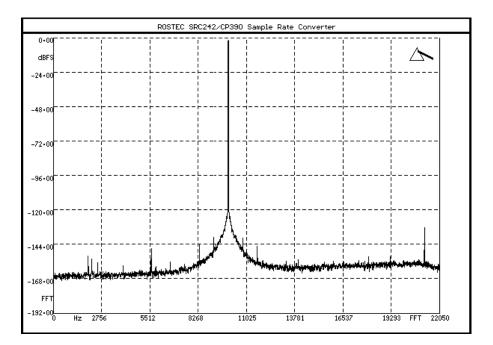
Input 10 kHz, -1 dBFs at 48 kHz
