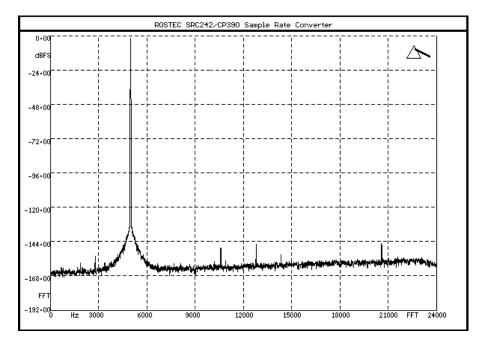
Input 5 kHz, -1 dBFs at 44.1 kHz
