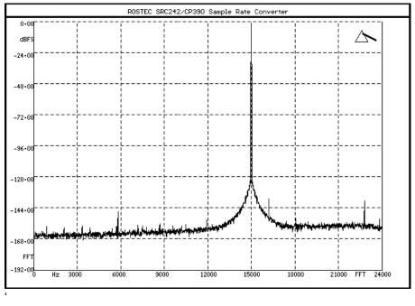
Input 15 kHz, -1 dBFs at 44.1 kHz Output 15 kHz, -1 dBFs at 48 kHz
