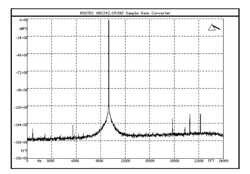
Input 10 kHz, -1 dBFs at 44.1 kHz
