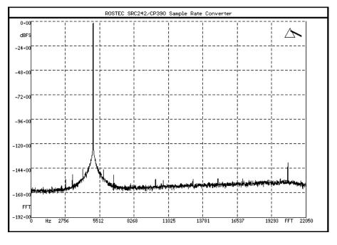
Input 5 kHz, -1 dBFs at 48 kHz
