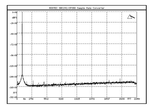
Input 1 kHz, -1 dBFs at 48 kHz
