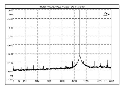
Input 15 kHz, -1 dBFs at 48 kHz Output 15 kHz, -1 dBFs at 44.1 kHz THD+N -117,11 dBFs, 20 Hz – 20 kHz unweighted
