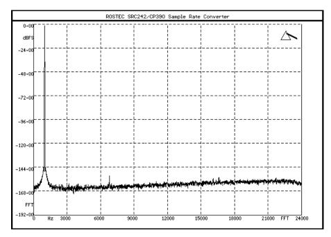
Input 1 kHz, -1 dBFs at 44.1 kHz
