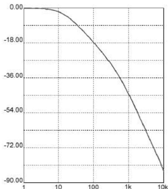
Jitter Attenuation dB vs. Frequency.
